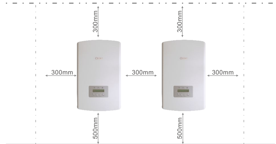
▲ Figure 4.1 Inverter Mounting clearance
