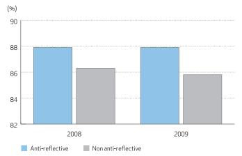
Performance ratio for REC modules with and without anti-reflective coating.
