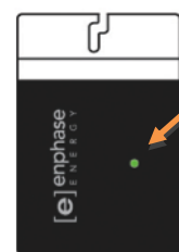
LED on underside of micro-inverter
