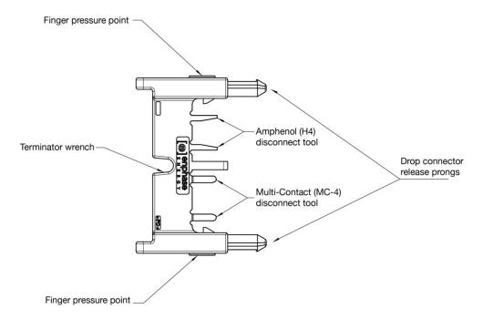
If the disconnect tool is not available, insert a #3 Phillips screwdriver into one hole, and rock that side of the drop connector out. Then, insert the screwdriver into the other hole and pull the connector out entirely.
