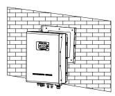
Fig.4 Hang inverter to mounting frame
