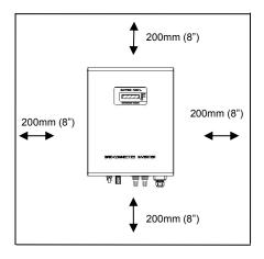
Fig.2 Installing minimum clearances around inverter
