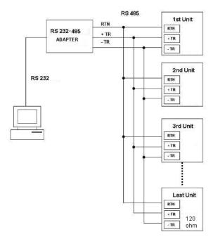
Fig.12 Multiple daisy-chain connection
