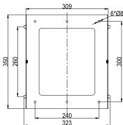
Fig.3 The size of mounting frame
