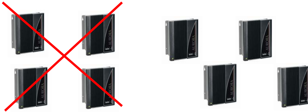
Fig.8 Aurora, recommended assembling
