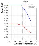
Fig. 2-9 Over-temperature Power Derating Curves (Charging)
