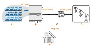
Fig. 2-1 Inverter Application in PV Power System
