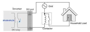
Fig. 9-1 DO Operation in Timer Control
