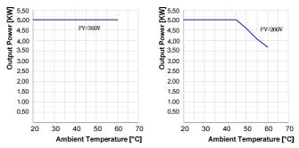
Fig. 2-7 Over-temperature Derating Curves of PV Power
