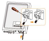
5. Fasten the swivel nut and connect the other end of the cable to the original edge of AC contactor.
