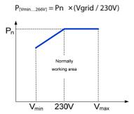
Fig. 2-10 Grid Under-voltage Derating
