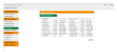
This interface is to set the related battery parameters. The following table describes the parameters explanation of "Other Lead-acid battery".
