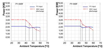
Fig. 2-8 Over-temperature Power Derating Curves (Discharging)
