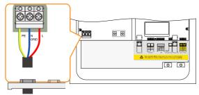
7. Fasten the swivel and connect the other end to the AC circuit breaker.
