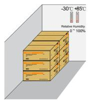
Fig. 3-4 Example of Inverter Storage
