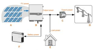
Fig. 2-2 Inverter Application in PV Energy Storage System
