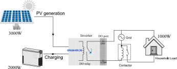
Fig. 9-3 DO Operation in Optimized Control
