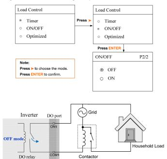
Fig. 9-2 DO Operation in ON/OFF Control
