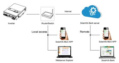
Fig. 5-6 Ethernet Connection with a Router
