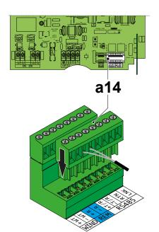
The connection and disconnection of the inverter to and from the grid can be controlled through an external control.
