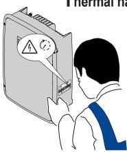
WARNING: removal of guards or covers is allowed only after the voltage has been removed; ; this is to let components cool down and allow any electrostatic charges and parasitic voltages to be discharged.
