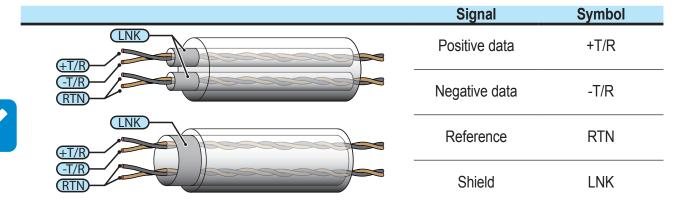
Shield continuity must be provided along the communication line using the SH terminal and must be grounded at a single point.
