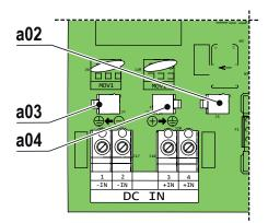
The grounding of the inputs **is negative configuration by default**. For the correct operation, some photovoltaic panels require the connection of the potential of the positive terminal to the earth terminal, or to have both of the input poles floating in regards to ground potential.
