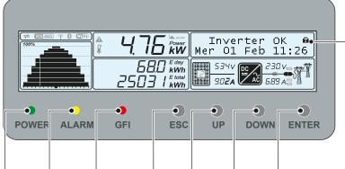
By pressing and holding the ENTER key, the cyclical display of the parameters can be:
