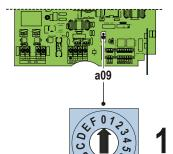
Before connecting the inverter to the distribution grid it is necessary to set the country standard by manipulating the two rotary switches <u>a09</u> and following the instructions in the table displayed in the relevant section.v
