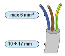
The cross-section of the AC line conductor must be sized in order to prevent unwanted disconnections of the inverter from the grid due to high impedance of the line that connects the inverter to the power supply point; In fact, if the impedance is too high, it causes an increase in the AC voltage that, on reaching the limit set by the country of installation, causes the inverter to switch off.
