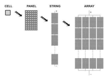
The current of each array must fall within the limits of the inverter.
