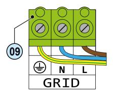
For all models you connect the AC output screw terminal block <sup>(9)</sup> by passing the cables through the AC cable gland <sup>(8)</sup>.
