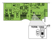
When using an RS-485 connection, if one or more inverters are added later to the system, you must remember to return to OFF position the switch of the termination resistance used of the inverter that was previously the last one of the system.
