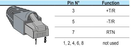
Use a connector with metal body to provide cable shield continuity!
