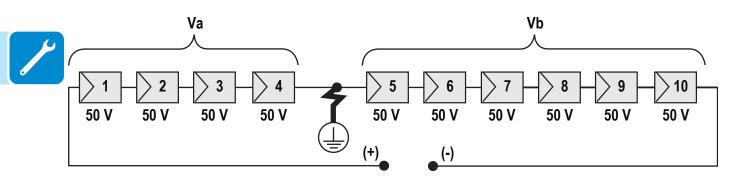
Va = voltage measured between + pole and 1 = 200V Vb = voltage measured between - pole and 1 = 300V In all measurements with 1, the ground of the inverter is indicated.
