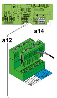
On the inverter there is a RS485 communication line, dedicated to connecting the inverter to monitoring devices or to carrying out "daisy-chain" ("in-out") connections of multiple inverters.
