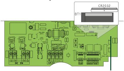
Back-up battery replacement procedure:
