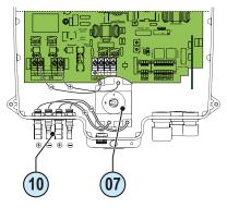
For the string connections it is necessary to use the quick fit connectors (multicontact or weidmüller) located on the bottom of the mechanism. The maximum numbers of input strings which can be connected is 2.
