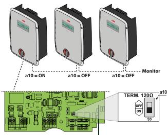
If a single inverter is connected to the monitoring system, activate the termination resistance of the communication line by switching switch <u>a10</u> (to ON position).
