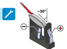
**3.** Install the new battery taking care to handle it with insulating gloves to ensure it is not discharged and respecting the polarity displayed on the communication board silkscreen
