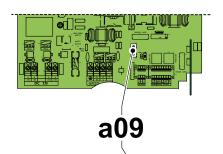
The inverter is configured using the rotary switches <u>a09</u>. Before turning the rotary switches, make sure the inverter is switched off! At the same time as the grid standard is set, the language of the display menus is also set.
