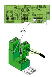
The inverter is equipped with a multifunction relay with configurable activation. It can be connected with normally open contact (being connected between the NO terminal and the common contact C) and with normally closed contact (being connected between the NC terminal and the common contact C).
