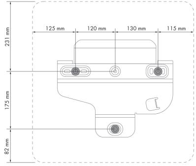
Figure 3: Position of the anchoring points
