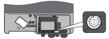
Figure 8: Positions of rotary switch C
