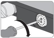
3. To deactivate communication via BLUETOOTH, set the rotary switch **C** to position **O** using a flatblade screwdriver (blade width: 2.5 mm). This will protect your PV system from unauthorized access.
