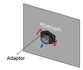
**Step 3** Connect SolarInfo Wireless or SolarInfo WiFi to the 5-pin terminal by plugging-in and tightening the cable gland.
