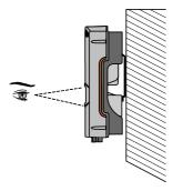
6. It is suggested that the inverter be installed vertically with upside up for good heat dissipation.
