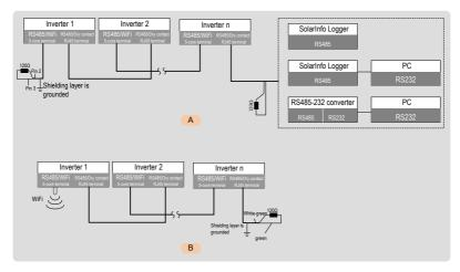
If the communication system is equipped with SolarInfo Logger, inverters may be dispatched by the power grid via dry contacts or remotely monitored via SolarInfo Bank.
