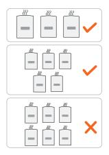
14. Do not install the inverter in a closed cabinet. Otherwise, the inverter will not operate normally.
