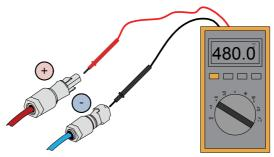
**Step 3** Plug the positive and negative DC connectors into corresponding terminals until there is an audible click.
