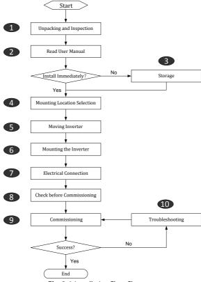
Fig. 3-1 Installation Flow Chart
