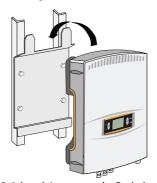
Fig. 5-4 Attach Inverter to the Backplate
