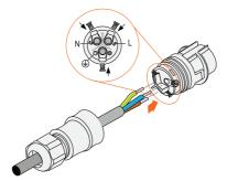
**Step 5:** Pull cables outward to check whether they are firmly installed.
