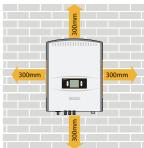
13. For multiple inverters installation, position the inverters side by side. For multi-row inverters installation, position the inverters in a staggered arrangement.
