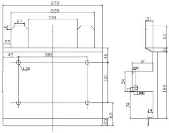
Fig. 5-1 Fastener(unit: mm)
