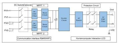
Fig. 2-5 Main Circuit Diagram of inverter
