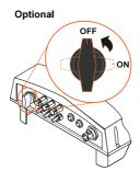
**Step 2** Check the connection cable of PV string for the correct polarity and that the open circuit voltage does not exceed the inverter input limit 550V, even under the lowest operating temperature. Refer to module specification supplied by module manufacturer for detailed information.
