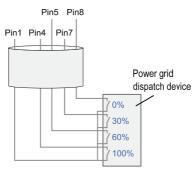
The connection procedures of the dry contacts to RJ45 terminal are the same as the RS485 connection to RJ45 terminal.
