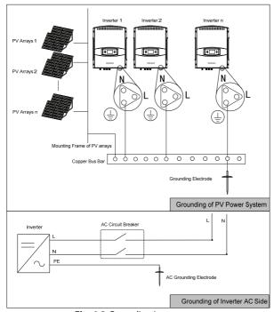
Fig. 6-3 Grounding Inverter
