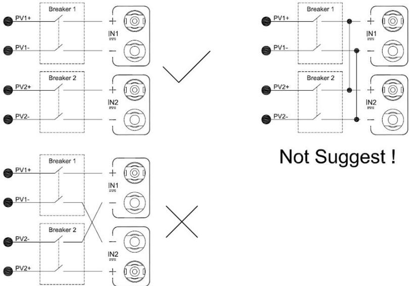
**Note:** Ensure that photovoltaic field voltage polarity matches the “+” and “-” symbols. Before connecting SUNTWINS inverters with the photovoltaic field, JFY-tech recommends to check, using a proper gauge, that the polarity value and the voltage allowed value between positive and negative contacts are correct.
