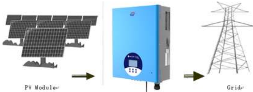
Figure 1 Principle of a PV Plant with ST series inverter
